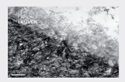
The transmission electron microscope (TEM) shows the interface image of CLEARFIL™ SE BOND.
