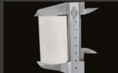
Carefully level the ring so that the top and bottom are perpendicular to the sides of the ring
