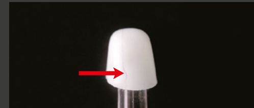
Crack is happened during grinding
