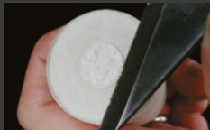
Remove the button of investment created by leveling cap
