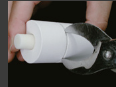
Final removal with a plaster nipper
